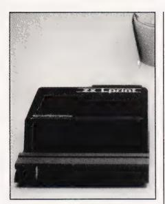
A close up of the ZX LPRINT from Euroelectronics. It's neat and compact but the edge connector PCB tracks are exposed (don't drop paperclips down the back of the Spectrum) and doesn't allow other peripherals to be connected — yet.
